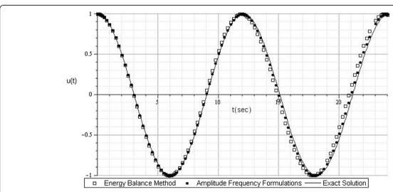
Figure 5 Comparison of energy balance method and amplitude-frequency formulation with exact solution when A=1,  $\lambda=0.95$ .
