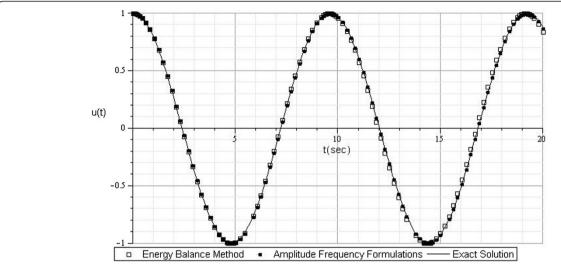
Figure 4 Comparison of energy balance method and amplitude-frequency formulation with exact solution when A = 1,  $\lambda = 0.75$ .
