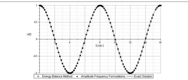
Figure 3 Comparison of energy balance method and amplitude-frequency formulation with exact solution when A = 1,  $\lambda = 0.5$ .
