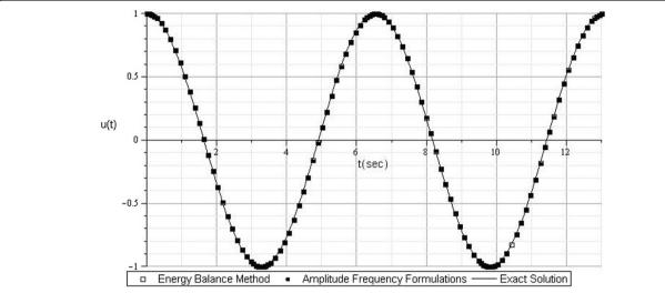
Figure 2 Comparison of energy balance method and amplitude-frequency formulation with exact solution when A = 1,  $\lambda = 0.1$ .
