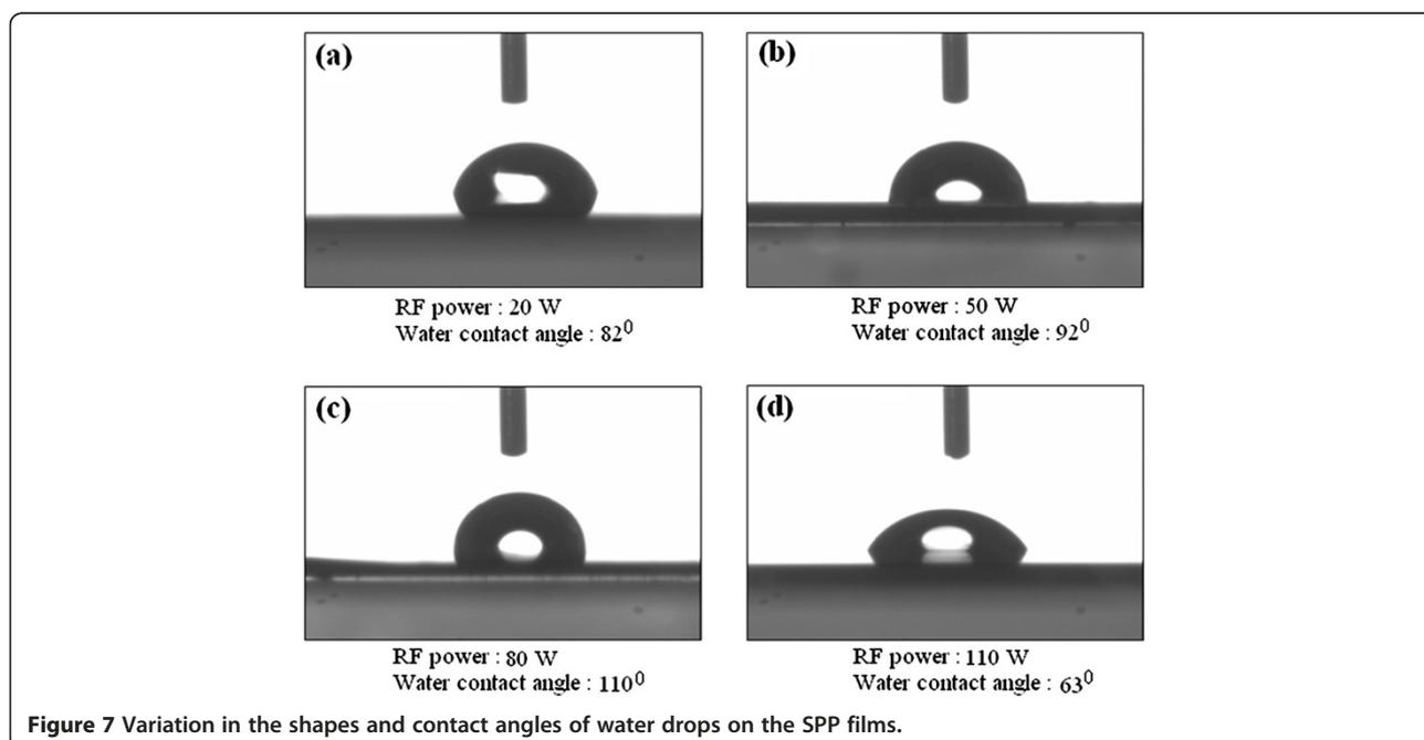
**Figure 7** Variation in the shapes and contact angles of water drops on the SPP films.
