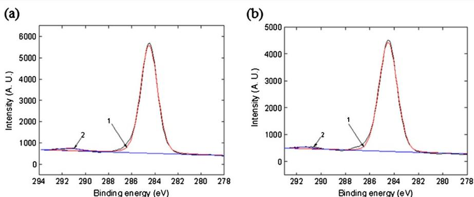
**Figure 6 Curve fit of the C1 peaks of the SPP films.** The films are deposited at RF powers of (a) 20 and (b) 110 W (1, C-C and/or C-H; 2, π - π\* shake-up satellite).
