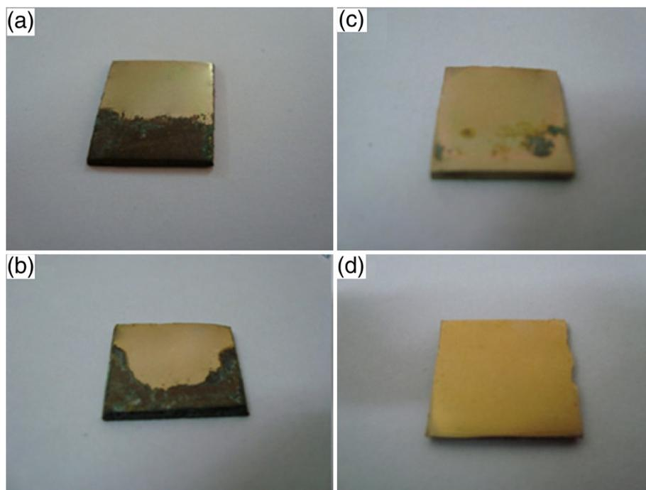
**Figure 19** Images showing visually observed corrosion tested surfaces of virgin bell metal and SPP films. (a) Virgin bell metal and SPP films deposited at RF powers of (b) 110, (c) 50 and (d) 80 W.
