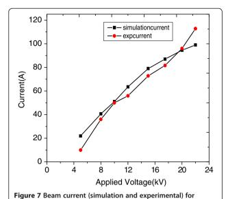
voltage variation from 5 to 22 kV at different axial locations. In all cases, the beam current is found to be minimum at z = 14.5 cm.
