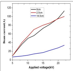
Figure 6 Beam current at different axial locations for different applied voltages.
