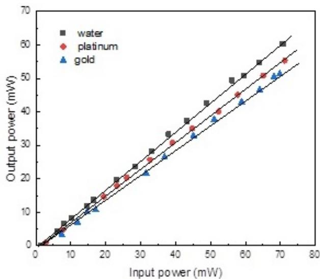
**Figure 3.** Transmittance measurement of the water, platinum nanoparticles and gold nanoparticles in the water.
