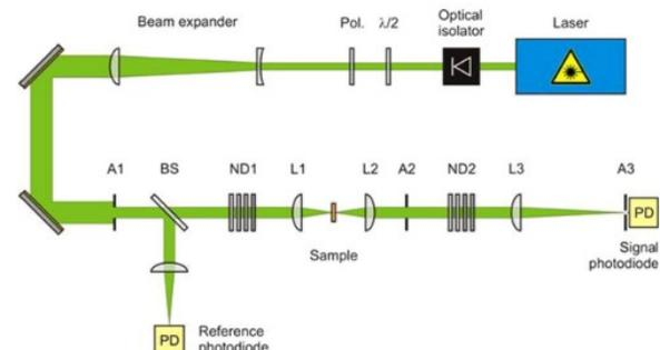
**Figure 4.** The closed Z-scan optical set up.
