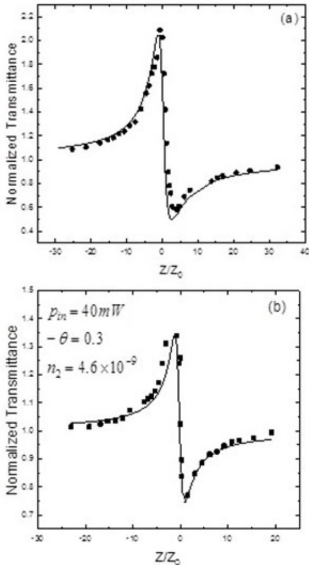
**Figure 5.** Experimental results of the normalized closed aperture Z-scan measurement of the (a) platinum nanoparticles and (b) gold nanoparticles in the water.
