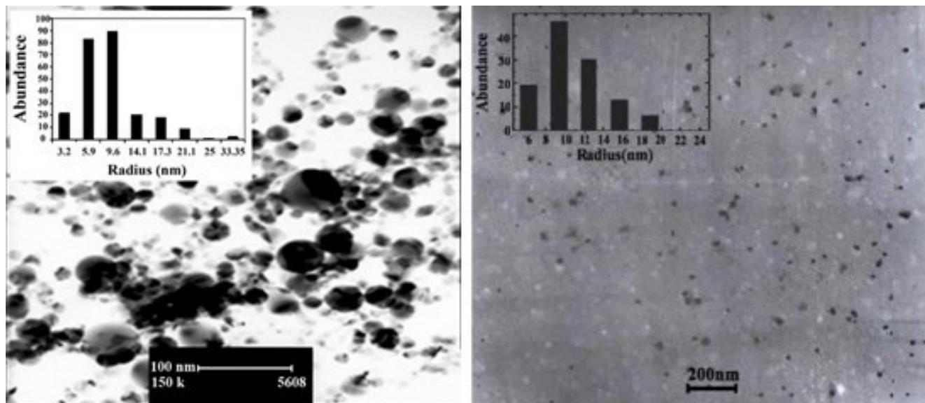
**Figure 2.** TEM images and size distribution of the (a) platinum and (b) gold nanoparticles in the water.
