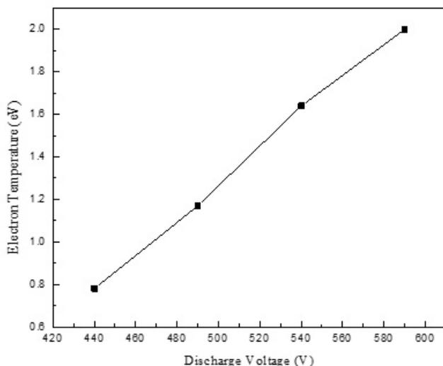
**Figure 4.** Variation in electron temperature with discharge voltage.
