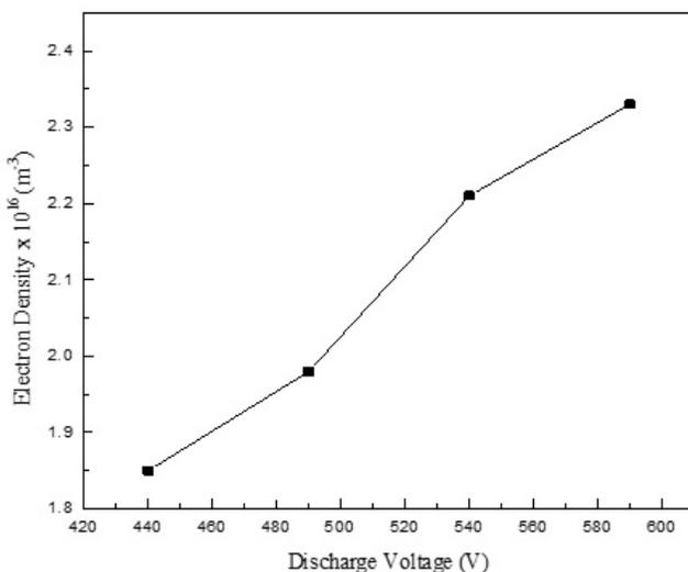
**Figure 5.** Variation in electron density with discharge voltage.
