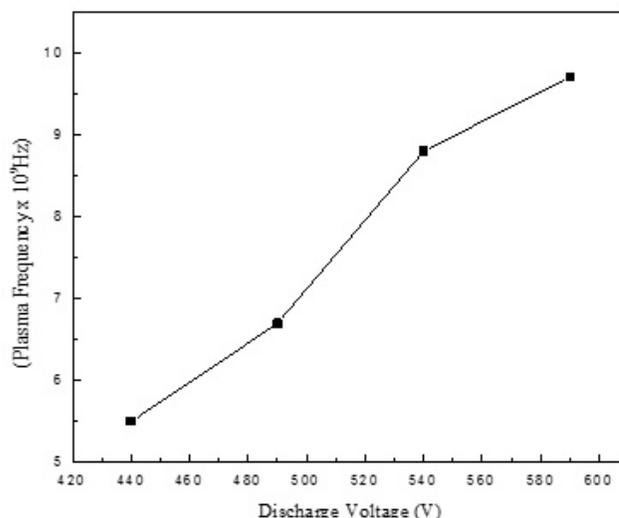
**Figure 6.** Variation in plasma frequency with Discharge voltage.
