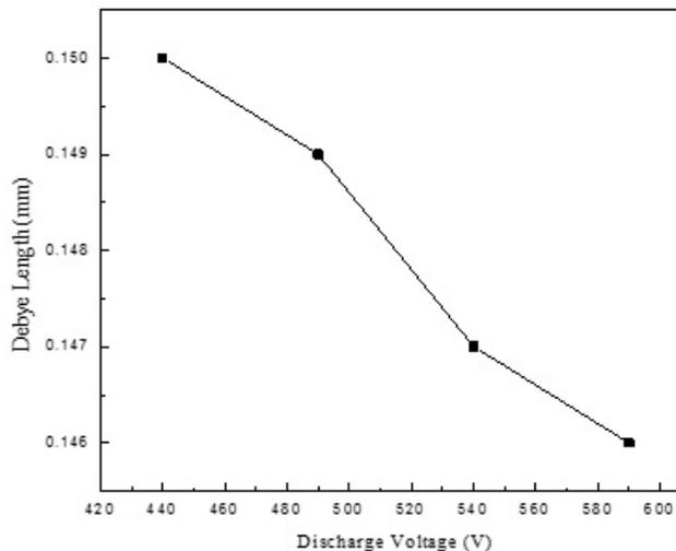
**Figure 7.** Variation in Debye length with discharge voltage.
