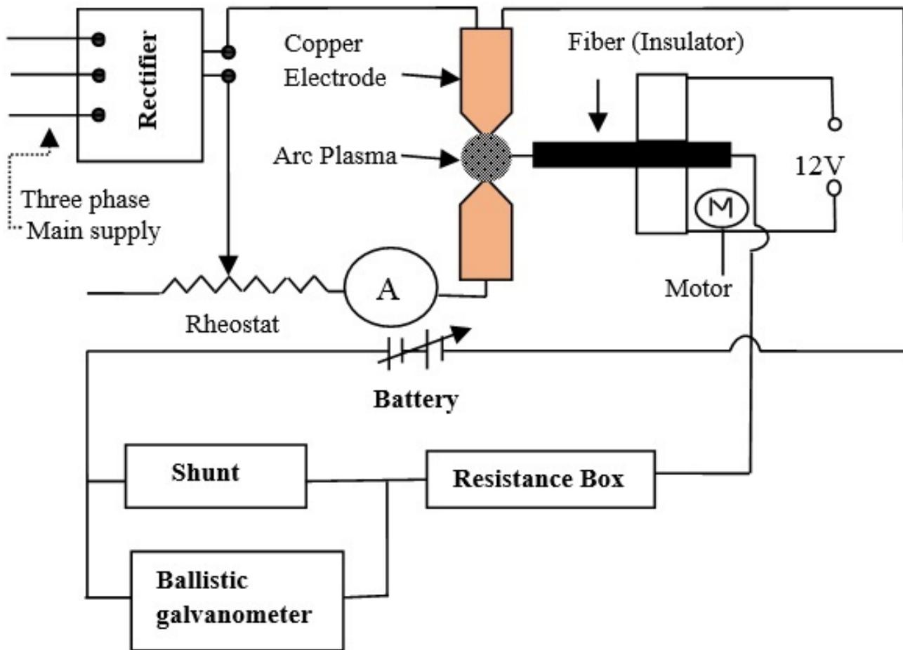
Figure 1. Basic circuit for single probe method.
