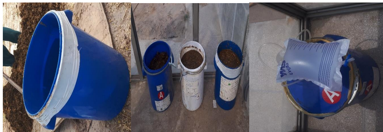
Fig. 2 Filling of homogenized composting material in the drums (20 L size) and completely sealing the drums for the composting and production of biogas
