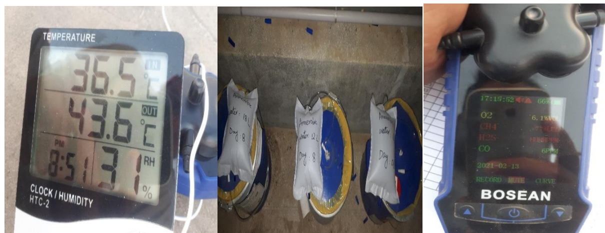
Fig. 3 Data recording for daily temperature, gas volume and greenhouse gasses emission
