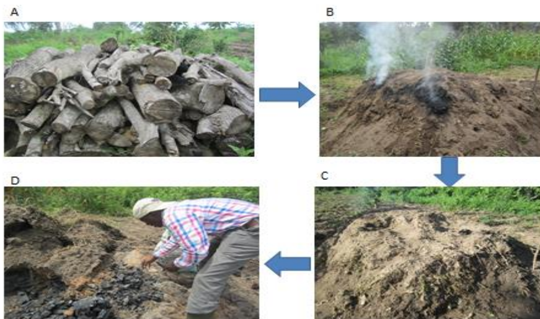
Fig. 2 Steps in local production of biochar from mango tree (A): Arrangement of logs for local pyrolysis. (B): Logs were covered with soil and fire was introduced from within to create anaerobic wood combustion under 1500 °C. (C): The process completed in the 7 th day. (D): Harvesting of the Biochar
