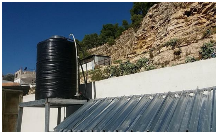
Fig. 2 The solar reactor which used in the treatment of OMW
