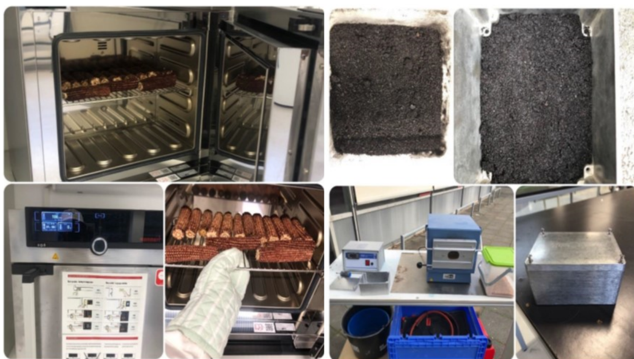
Figure 1. Preparation of corncob and pyrolysis process.
