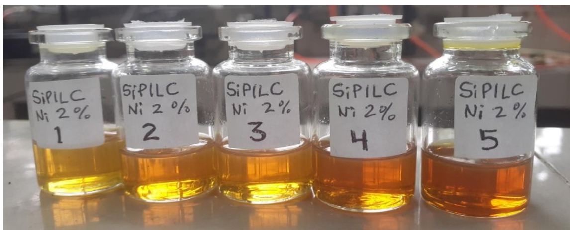
Fig. 13. Photo of a liquid product resulting from the hydrocracking of HDPE plastic with a Ni 2%/SiPILC catalyst with variations of catalyst reuse
