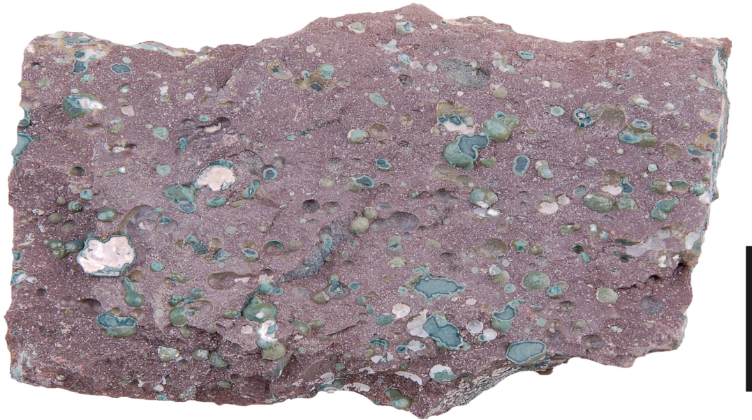
Figure 6. Mafic rock (melaphyre) with typical amygdaloid texture. Inside amygdales, there are usually quartz or calcite infilled with blue-green secondary minerals. Scale bar = 5 cm. Courtesy Municipal Museum Nová Paka, photo by V. Mencl.
