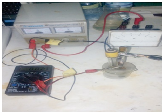
Figure 1. Pictorial representation of an electrodeposition setup.
