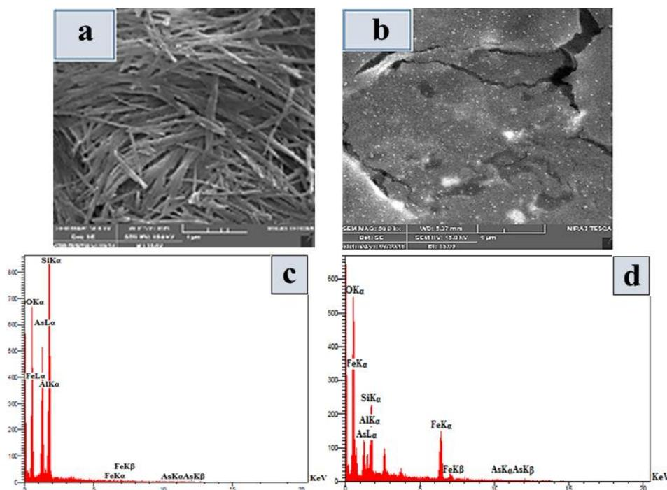
Fig 2. (a) SEM result of S2 sample (Arsenic polluted sepiolite), (b) SEM result of ES2 sample (polluted soil after acid washing), (c) EDX spectra of S2 sample, (d) EDX spectra of ES2 sample
