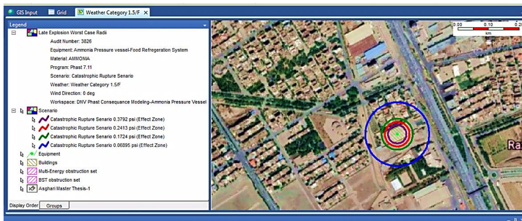
Fig 9. The blast wave caused by the explosion of the ammonia tank of the ammonia refrigeration system
