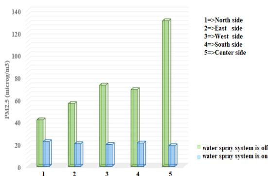
Figure 3. PM2.5 parameter when water spraying system is off and on
