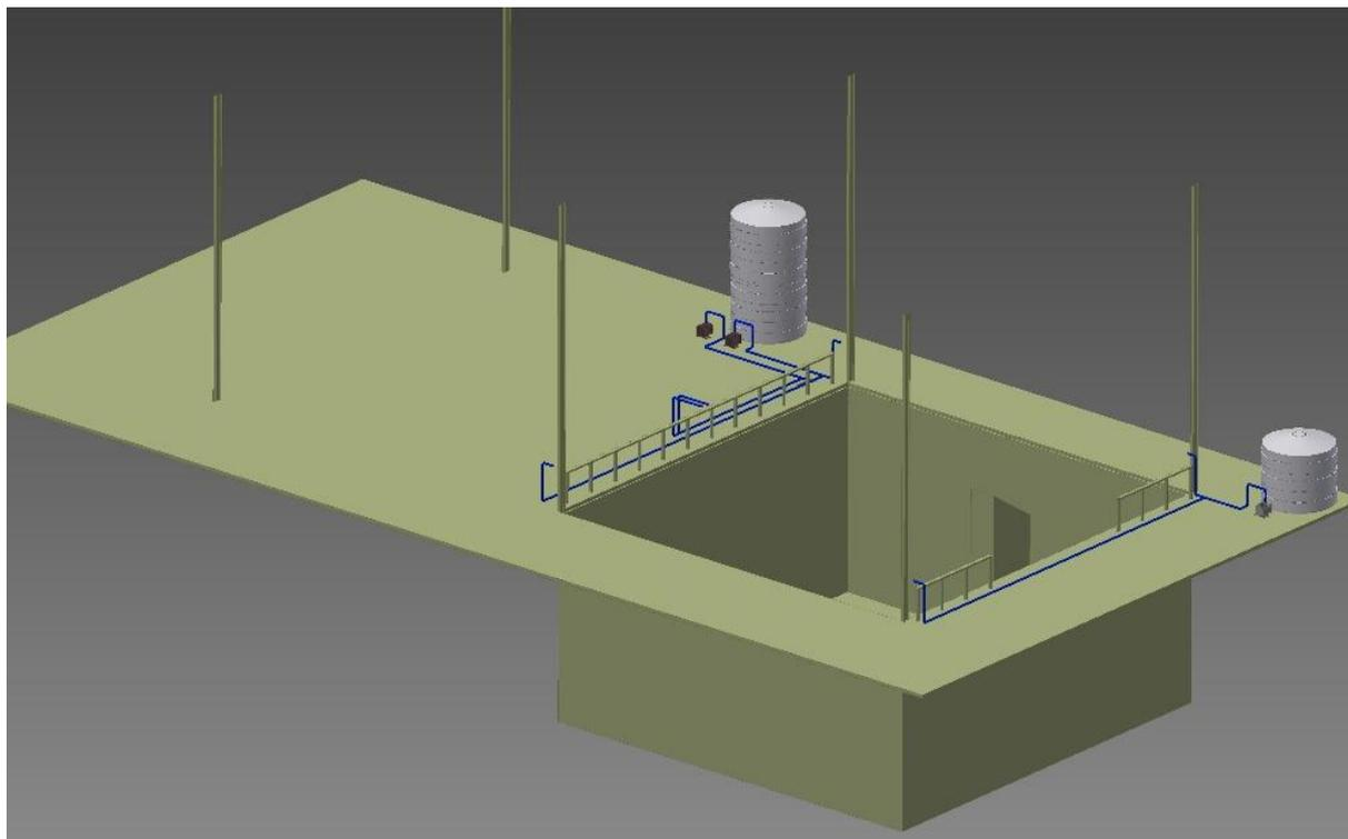
Figure 2. Side view of water spraying system in gyratory crusher
