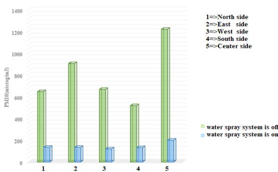
Figure 4. PM10 parameter when water spraying system is off and on
