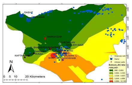
Figure 5. Spatial distribution of EC l value in Jajarm region, Iran, processed by ArcGIS® 10.3 shows that the EC value is high in the region (in red colour)
