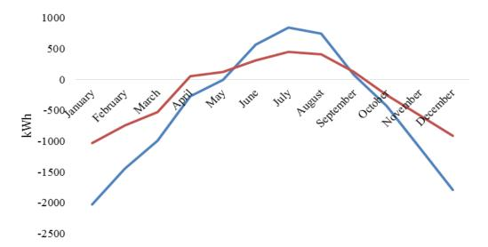
Figure 9. Heat transfer from the ceiling (Red line: optimal mode - Blue line: base mode)
