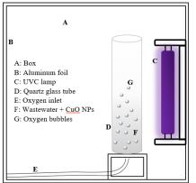
Fig. 2: Schematic representation of a photocatalytic reactor
