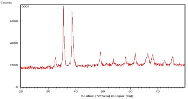
Fig. 5: XRD pattern of the synthesized CuO nanoparticles
