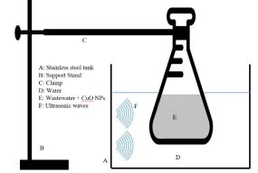
Fig. 3: Schematic representation of a sonocatalytic reactor
