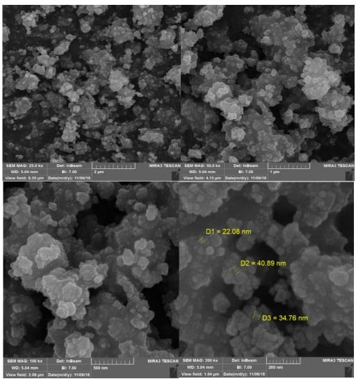
Fig. 6: SEM images of CuO nanocrystals with the scales of 1 µm, 2 µm, 200 nm, and 500 nm
