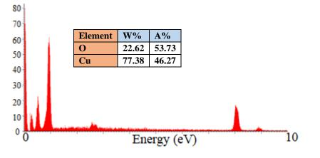
Fig. 7: Energy dispersive x-ray spectrum of CuO nanoparticles
