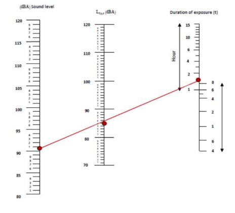
Fig. 6- Nomogram of calculating the allowable duration of exposure to sound for athletes in bodybuilding clubs in Mashhad (Source: Research finding)
