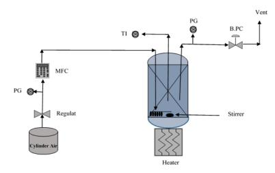
Fig. 1- Schematic of a laboratory reactor system for catalytic wet air oxidation; equipment: air cylinder, B.PC regulator, mass flow controller (MFC), batch reactor, heater, stirrer, pressure gauges (PG) and temperature indicator (TI) and controller
