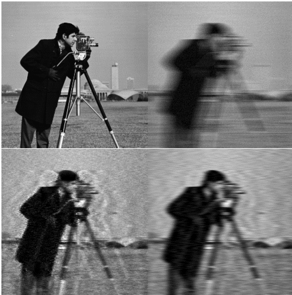
Figure 1. (a) Original image; (b) Motion blurred image with blur extend = 31, SNR = 30 dB; (c) Lucy-Richardson method, PSNR = 19.98; (d) regularized filter, PSNR = 20.06.
