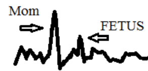
Figure 2. An ECG signal includes both the mother and the fetus [4].
