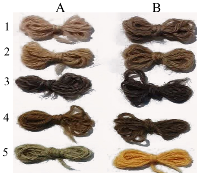
Figure 1. Fiber colors with different mordants by L/R = 30. A: Oleander flower, B: Bougainvillea flower, 1: No mordant, 2: Aluminum mordant, 3: Iron mordant, 4: Copper mordant, 5: Tin mordant.
