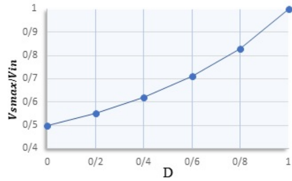
Figure 6. Normalized switch voltage stress vs. Duty Cycle.
