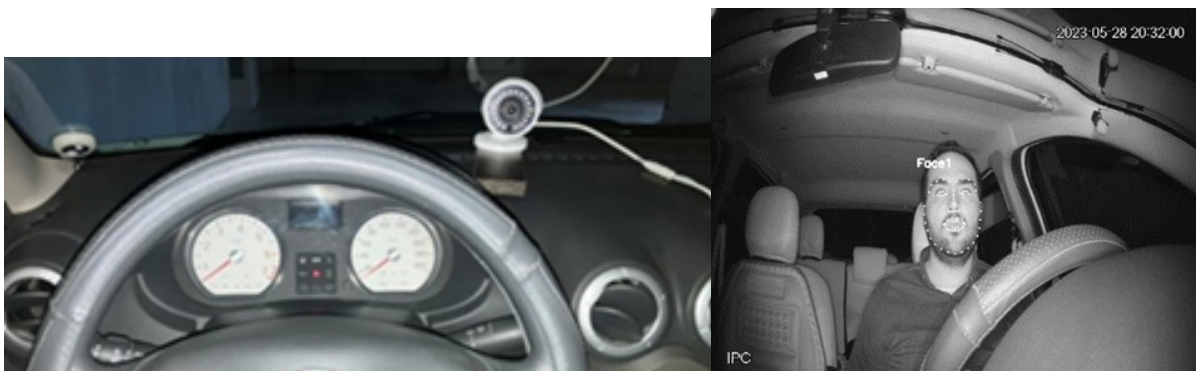
Figure 2. (a) Recommended camera mounting location, (b) Image acquired from the recommended mounting position.
