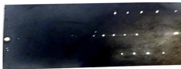
Figure 5. a-axis 15° oscillation photograph of a melt grown oscillation photograph of a melt-grown Ga-doped crystal, showing reflections of the most polytype 4H.
