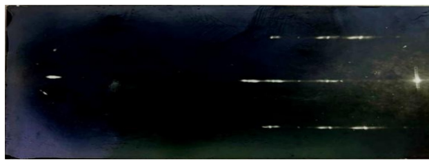
Figure 8. a-axis 15° oscillation photograph of a melt-growth Cl doped crystal, showing reflections of the most common polytype 4H, accompanied by 'streaking'; some extra diffuse reflections are also present.
