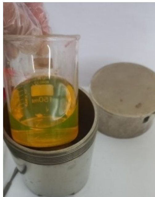
Figure 1. Citric acid solution obtained from lemons, which is placed in an autoclave.
