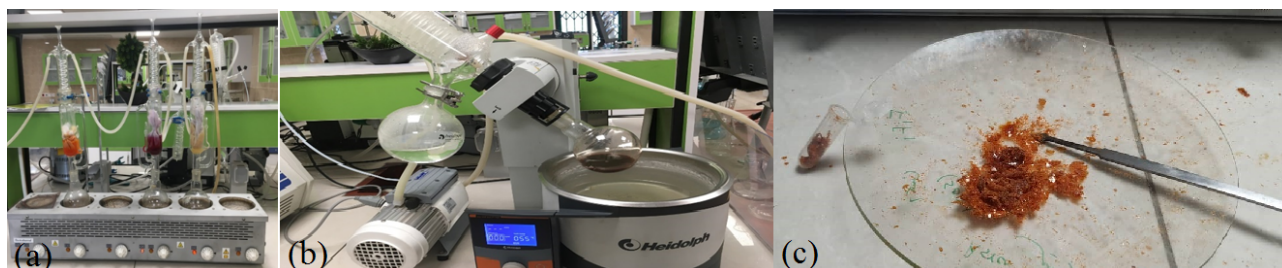
Figure 1. Preparation of the plant and its extraction, (a) Soxhlet apparatus, (b) rotary apparatus, (c) drying glass dishes and pre-sterilized microtubes.
