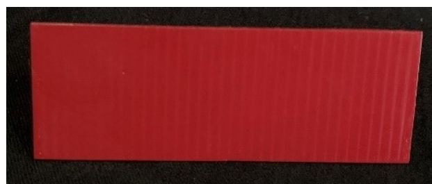
Figure 4. Grooved painted steel piece.
