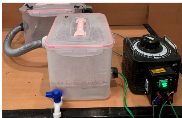
Figure 5. Dew formation test set-up.
