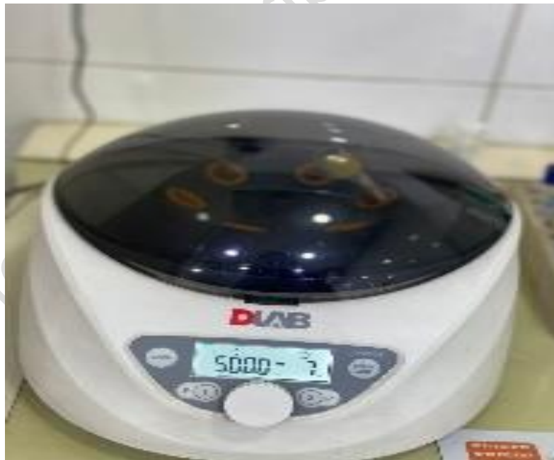
Figure 2 :Centrifugation process used to separate serum from whole blood samples.
