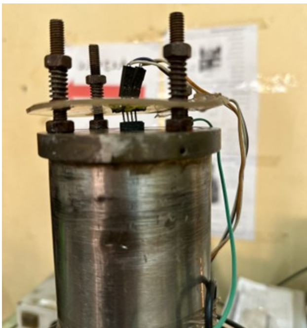
Figure 3. Photograph of the sample mounted inside the cryogenic measurement system.
