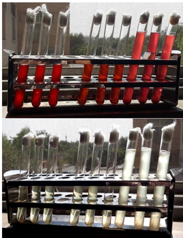
Figure 7. Images of tubes before (up) and after (down) subjection to the MPN test.
