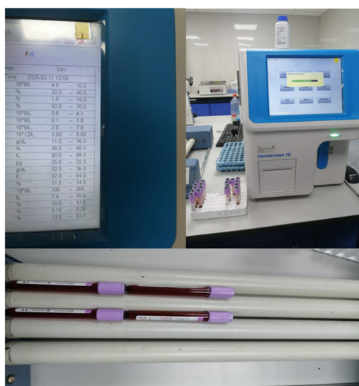
Figure 1. Hema screen 18 was used to measure some blood parameters like White blood cell (WBC), red blood cell (RBC), and platelet count (PLT) before and after exposure.
