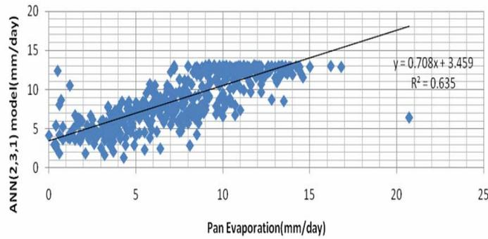
Fig. 7. Comparison of Daily Pan Evaporation with Different ANN (2-3-1) Model
