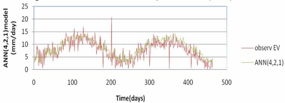
**Fig. 5.** Modeled and Measured Evaporation ANN (4-2-1)
