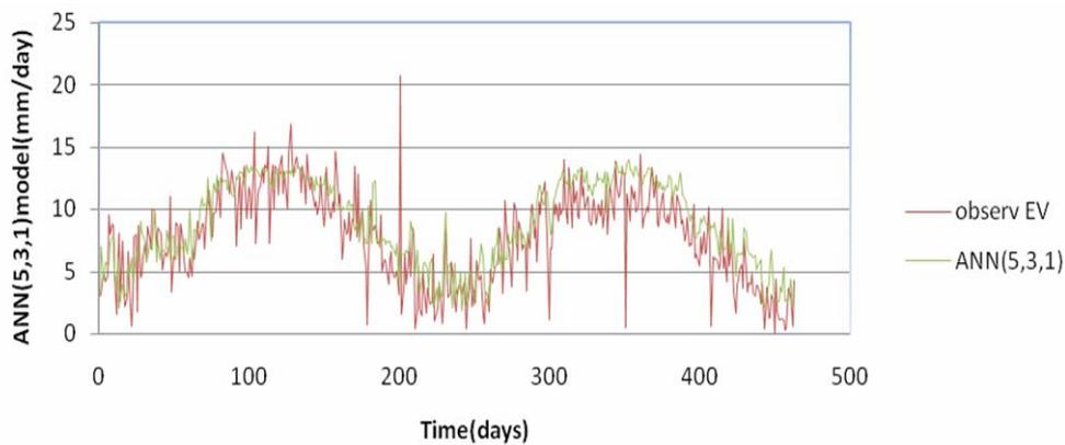
**Fig. 1. Modeled and Measured Evaporation ANN (5-3-1)**
