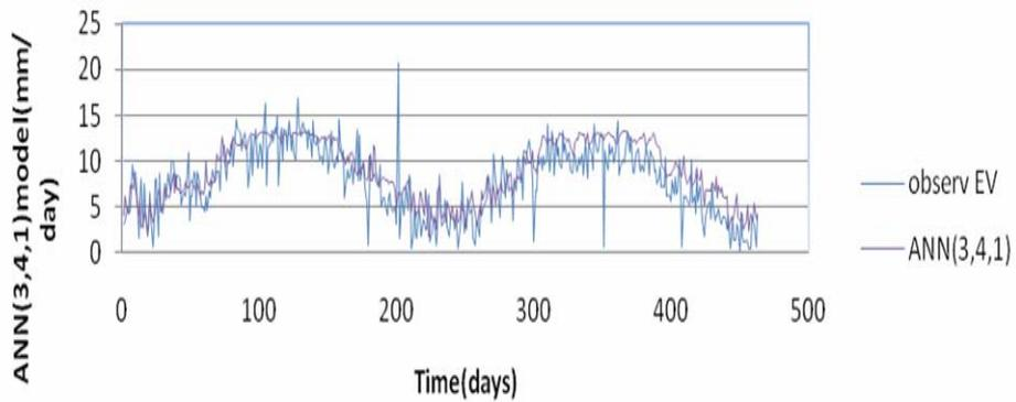
**Fig. 4.** Modeled and Measured Evaporation ANN (3-4-1)
