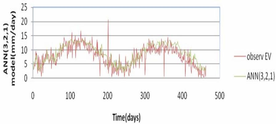
**Fig. 3.** Modeled and Measured Evaporation ANN (3-2-1)
