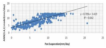
Fig. 9. Comparison of daily Pan Evaporation with Different ANN (3-4-1) Model
