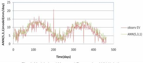
Fig. 1. Modeled and Measured Evaporation ANN (5-3-1)
