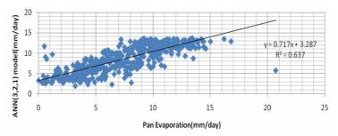
Fig. 8. Comparison of Daily Pan Evaporation with Different ANN (3-2-1) Model
