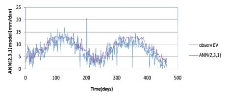
Fig. 2. Modeled and Measured Evaporation ANN (2-3-1)
