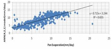
Fig. 10. Comparison of Daily Pan Evaporation with Different ANN (4-2-1) Model
