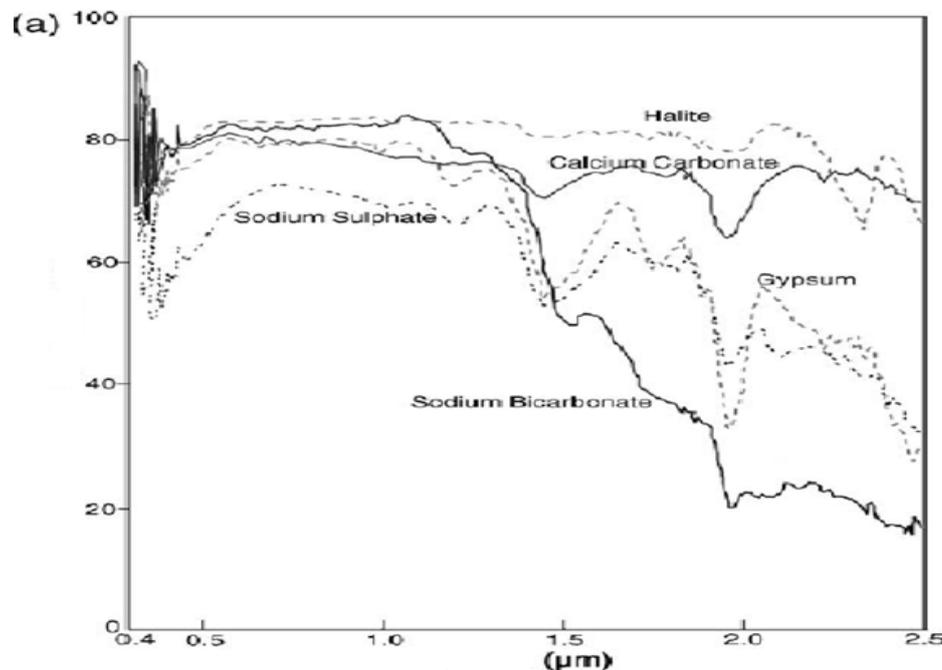
**Fig. 1.** Plaster range ( $\text{CaSO}_4 \cdot 2\text{H}_2\text{O}$ ), halite ( $\text{NaCl}$ ), calcium carbonate ( $\text{CaCO}_3$ ), sodium bicarbonate ( $\text{NaHCO}_3$ ) and sodium sulphate ( $\text{Na}_2\text{SO}_4$ ) in the visible, near infrared and middle area (0/4-2/5 nm) are measured by (GER 3700) Spectroradiometer (Howari *et al.*, 2002).
