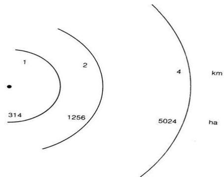
**Fig. 7.** The area of land within a given radius of the water point varies as the square of the distance from the water. The black dot in this diagram represents the location of the watering place.
