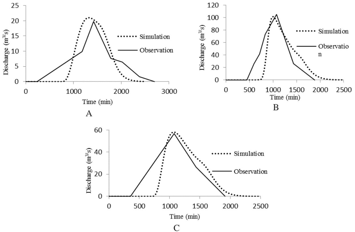
**Fig. 5.** Observed and simulated flood hydrographs in Tamar station (used for calibration) A) 11/6/1997 B) 5/30/1998 C) 9/11/1998
