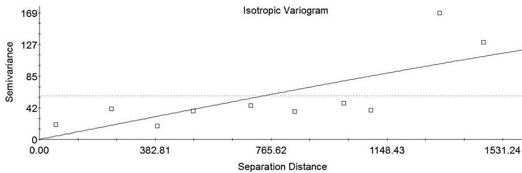
Spherical model ( $C_0 = 0.1000$ ;  $C_0 + C = 201.1000$ ;  $A_0 = 3798.00$ ;  $r_2 = 0.72$ ;  $RSS = .9784$ )
