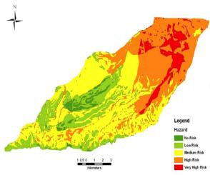
**Fig. 3.** Classified flood occurrence probability map of Gilard using AHP method
