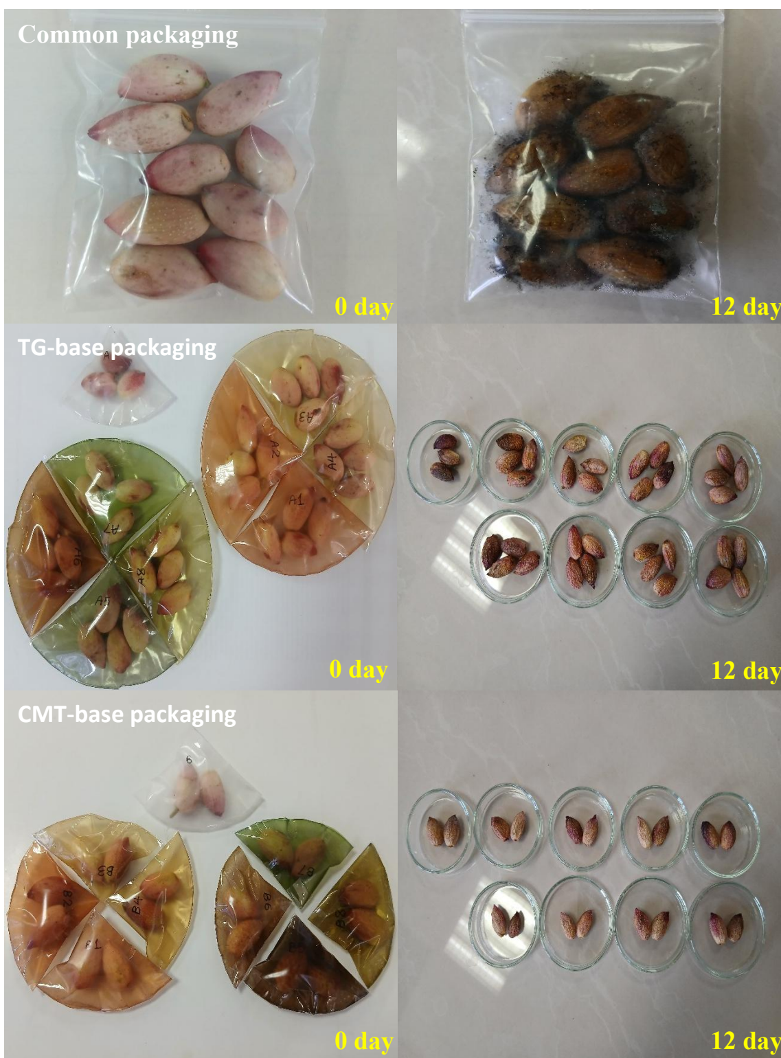
Figure 9. Packaging of raw pistachios using conventional plastic films and TG/CMT-based edible films containing biogenic nanoparticles and plant extracts. The active edible films significantly improved the preservation quality and extended the shelf life of pistachios during storage
