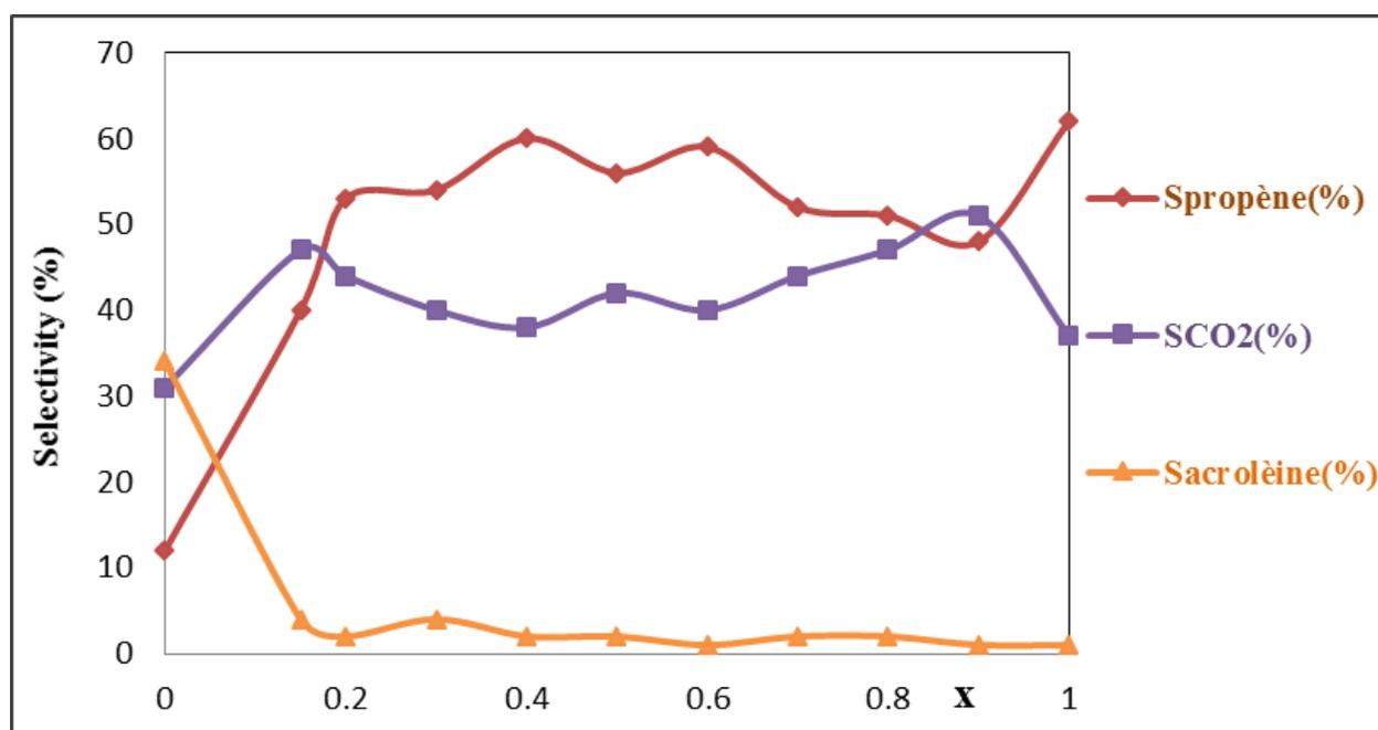
**Fig. 7.** Evolution of the Selectivity to propylene propelene, acrolein, and CO<sub>2</sub> with different vanadium Concentrations in the propane ODH. Reactions conditions: T = 480 °C, C<sub>3</sub>H<sub>8</sub>/O<sub>2</sub>/He = 10/10/80 (mol%).
