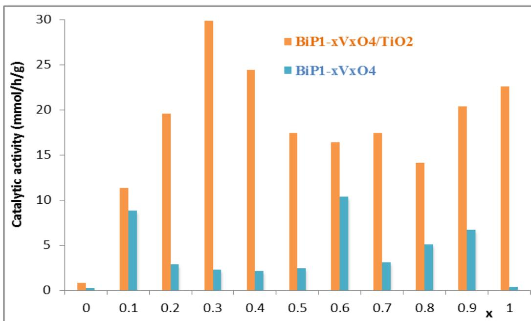
**Fig. 6.** Comparison of the global activity of BiP<sub>1-x</sub>V<sub>x</sub>O<sub>4</sub> and BiP<sub>1-x</sub>V<sub>x</sub>O<sub>4</sub>/TiO<sub>2</sub> in methanol oxidation. Reactions conditions: T = 250 °C, CH<sub>3</sub>OH/O<sub>2</sub>/He = 7.1/15.5/77.4 (mol%).
