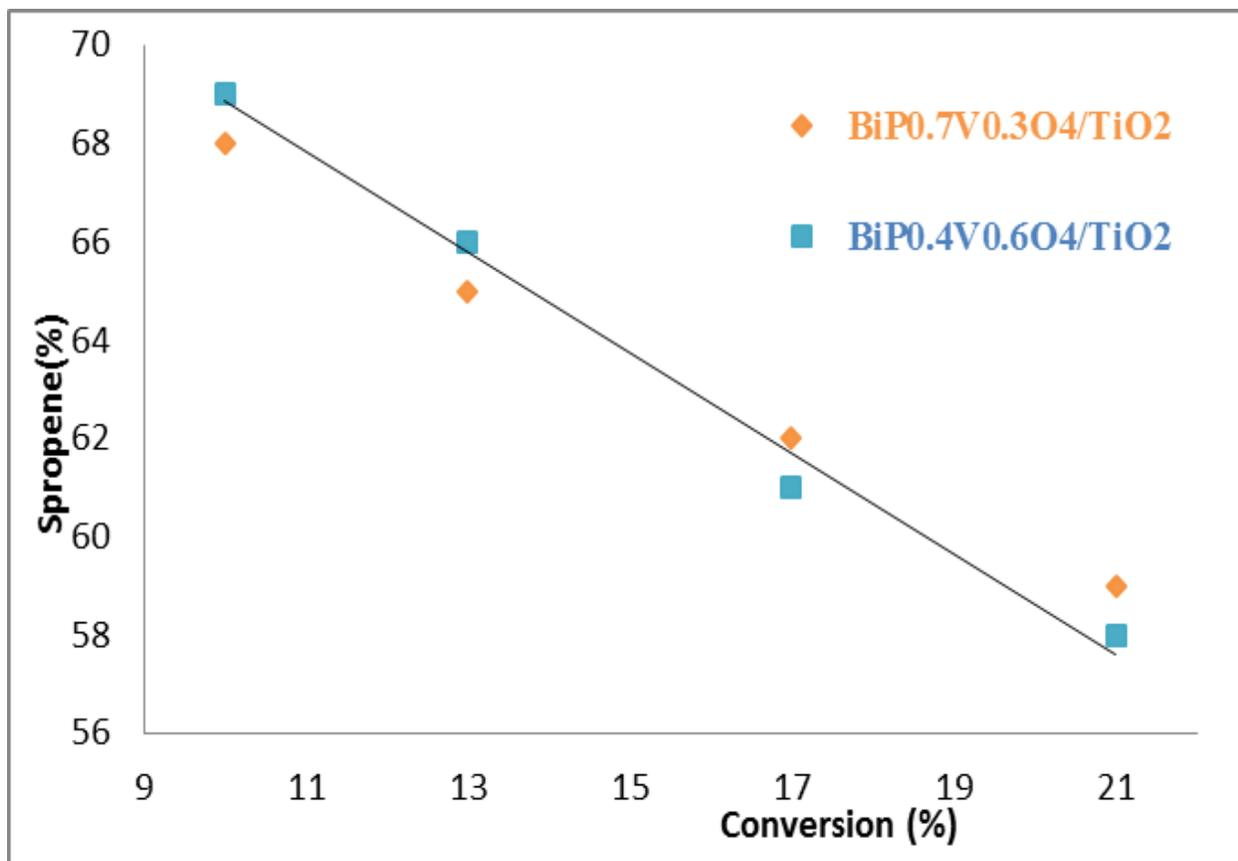
**Fig. 9.** Evolution of the selectivity for propene as a function of the conversion for Catalysts BiP<sub>0.7</sub>V<sub>0.3</sub>O<sub>4</sub>/TiO<sub>2</sub> and BiP<sub>0.4</sub>V<sub>0.6</sub>O<sub>4</sub>/TiO<sub>2</sub>. Reactions conditions: T = 480 °C, C<sub>3</sub>H<sub>8</sub>/O<sub>2</sub>/He = 10/10/80 (mol%).
