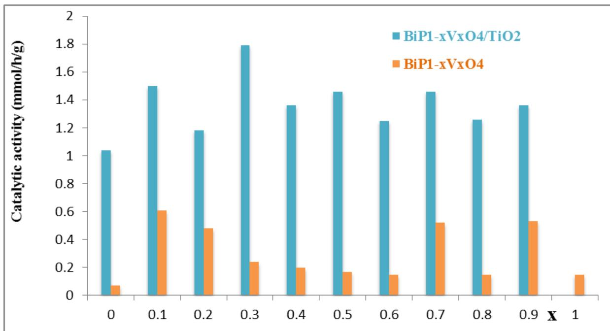
**Fig. 8.** The comparison of the global activity of BiP<sub>1-x</sub>V<sub>x</sub>O<sub>4</sub> and BiP<sub>1-x</sub>V<sub>x</sub>O<sub>4</sub>/TiO<sub>2</sub> in the ODH of propane reaction. Reactions conditions: T = 480 °C, C<sub>3</sub>H<sub>8</sub>/O<sub>2</sub>/He = 10/10/80 (mol%).
