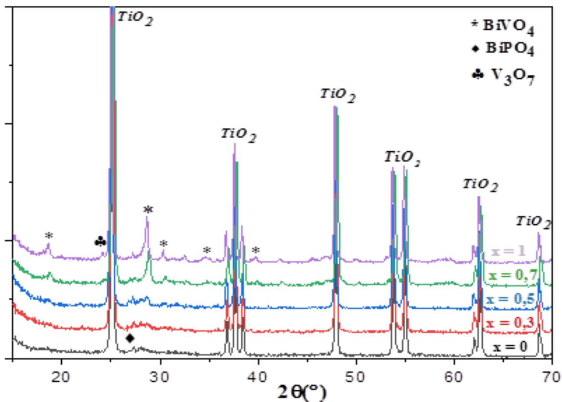
Fig. 1. XRD patterns of BiP<sub>1-x</sub>V<sub>x</sub>O<sub>4</sub>/TiO<sub>2</sub> catalysts.
