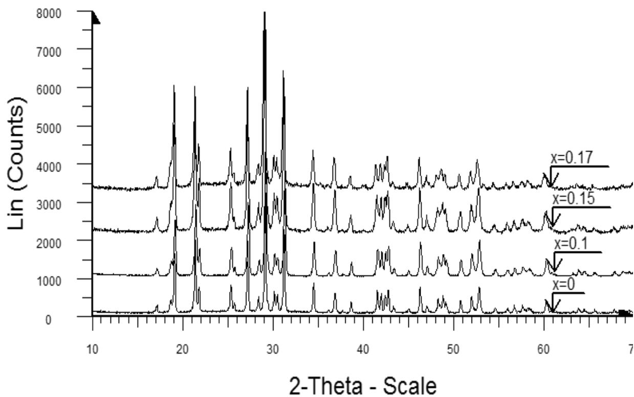
Fig. 2. X-ray diffraction spectra of unsupported BiP<sub>1-x</sub>V<sub>x</sub>O<sub>4</sub> catalysts isotype to BiPO<sub>4</sub> [22–26]
