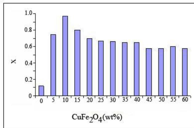
**Fig. 1.** Effect of composition of photocatalyst (wt.% CuFe<sub>2</sub>O<sub>4</sub> in mixture of CuFe<sub>2</sub>O<sub>4</sub> and CP) on photocatalytic degradation of AR206 after 120min.
