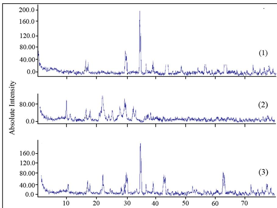
**Fig. 2.** XRD pattern of (1) raw  $\text{CuFe}_2\text{O}_4$  (2) CP (3) 10 wt.%  $\text{CuFe}_2\text{O}_4/\text{CP}$  prepared by the (SSD) method after calcination in air at  $450^\circ\text{C}$  for 5 h.
