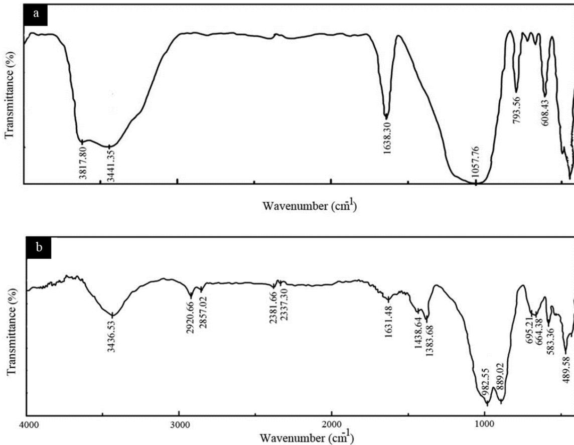
Fig. 4. (a) IR spectra of raw CP (b) CuFe<sub>2</sub>O<sub>4</sub>.
