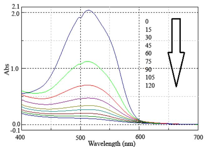
Fig. 5. UV-Vis spectra of AR206 (90 ppm) in aqueous photocatalyst dispersion with concentration of 60 ppm, irradiated with a mercury lamp light at pH = 4, T = 298 K, at: t = 0, 15, 30, 45, 60, 75, 90, 105, 120 min.
