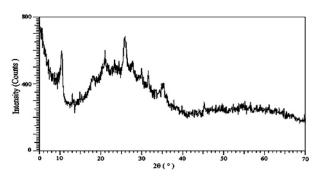
Fig. 4. XRD patterns of PW<sub>12</sub>@V-MCF.
