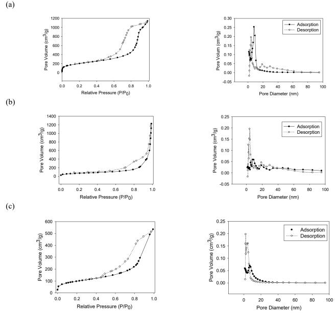
Fig. 5. (Right): N<sub>2</sub>-adsorption-desorption isotherms and, (Left): isotherm patterns of pore size distributions of (a) MCF; (b) V-MCF.
