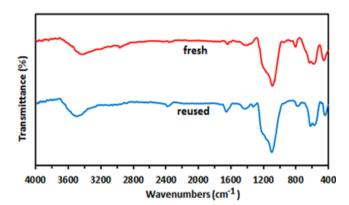
**Fig. 9.** The FT-IR spectra of fresh catalyst (Fe<sub>3</sub>O<sub>4</sub>@SiO<sub>2</sub>-AQ) and that reused six times.
