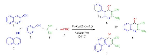
Scheme 3. Fe<sub>3</sub>O<sub>4</sub>@SiO<sub>2</sub>-AQ as a hybrid nanocatalyst for efficient synthesis of 4*H*-chromene derivatives.
