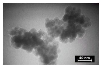
Fig. 3. TEM image of Fe<sub>3</sub>O<sub>4</sub>@SiO<sub>2</sub>-AQ nanoparticles.
