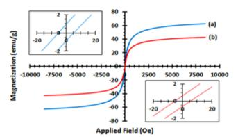
Fig. 7. The Magnetic hysteresis loops of (a)  $Fe_3O_4$  MNPs and (b)  $Fe_3O_4@SiO_2-AQ$ .
