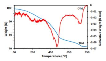
**Fig. 6.** The TGA-DTA curves of Fe<sub>3</sub>O<sub>4</sub>@SiO<sub>2</sub>-AQ nanoparticles.
