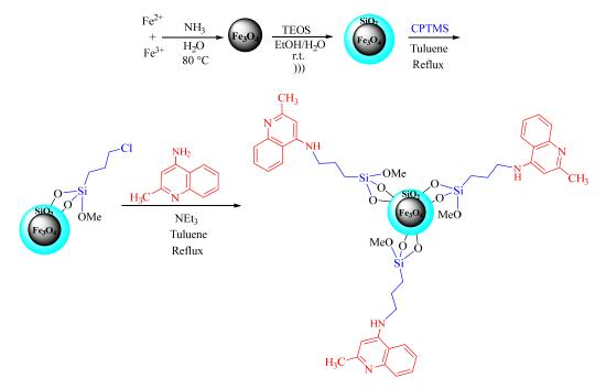
Scheme 2. Schematic steps for preparation of novel basic hybrid nanomaterial (Fe<sub>3</sub>O<sub>4</sub>@SiO<sub>2</sub>-AQ).
