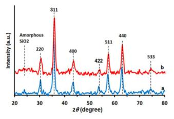
Fig. 5. The XRD patterns of (a)  $Fe_3O_4$  MNPs and (b)  $Fe_3O_4@SiO_2-AQ$ .
