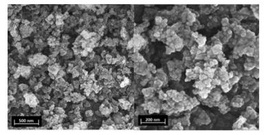
Fig. 2. FE-SEM images of Fe<sub>3</sub>O<sub>4</sub>@SiO<sub>2</sub>-AQ nanoparticles.
