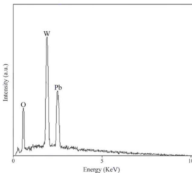
**Fig.4.** EDS spectrum of PbWO<sub>4</sub> nanostructures.
