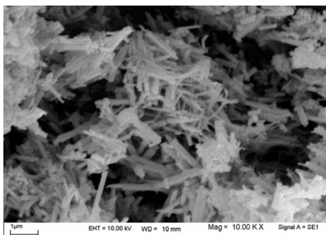
**Fig. 2.** SEM images of PbWO<sub>4</sub> nanostructures.
