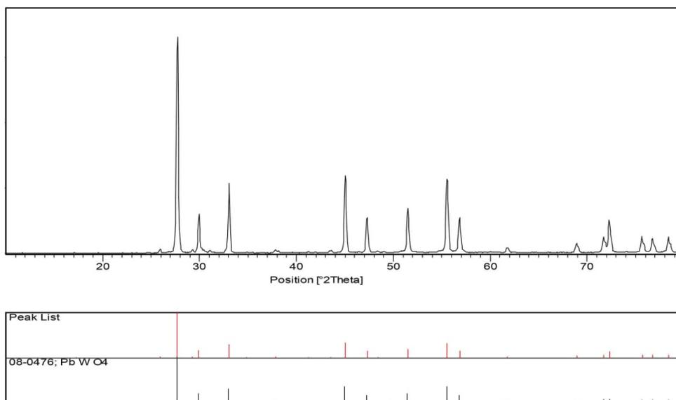
**Fig. 1.** XRD pattern of PbWO<sub>4</sub> nanostructures.
