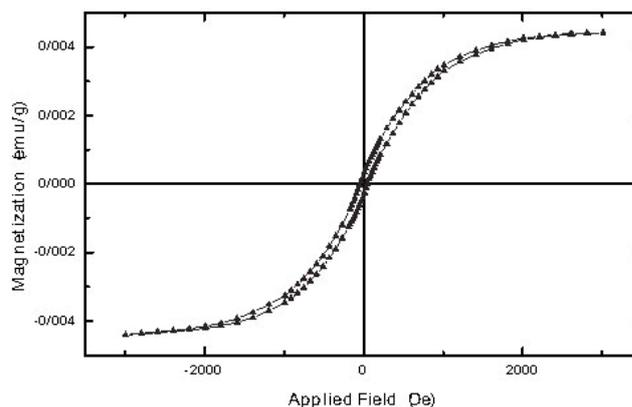
**Fig 3.** VSM curve of PbWO<sub>4</sub> nanostructures.
