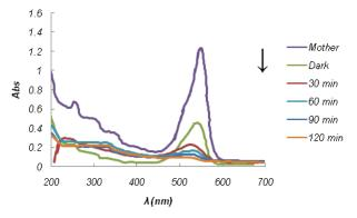
**Fig. 7.** Photodegradation of RB on bare ZnO/SiO<sub>2</sub> photocatalyst at pH=6.
