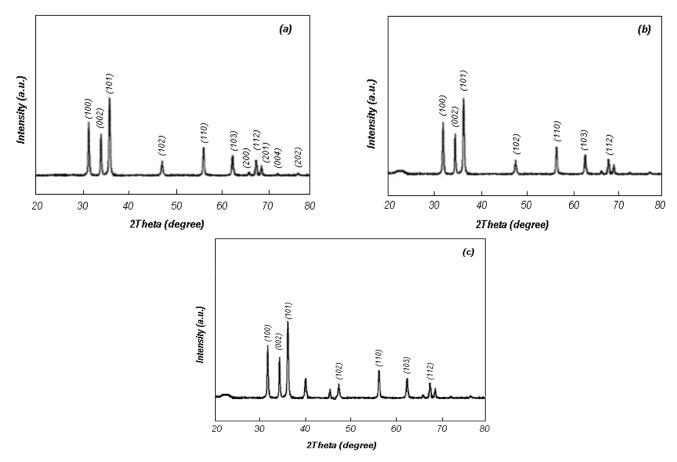
Fig. 1. XRD patterns of (a) ZnO, (b) ZnO/SiO<sub>2</sub>, and (c) Pt - ZnO/SiO<sub>2</sub> samples.
