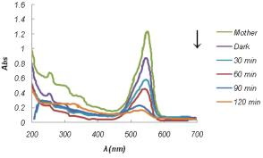
**Fig. 5.** Photodegradation of RB on bare ZnO/SiO<sub>2</sub> photocatalyst at pH=4.
