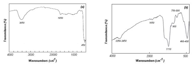
Fig. 2. FT-IR spectra of (a) ZnO and (b) ZnO/SiO<sub>2</sub> samples.
