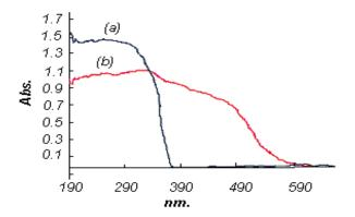
Fig. 10. UV-Vis Diffuse Reflectance Spectra of (a) ZnO/SiO<sub>2</sub>, and (b) Pt-ZnO/SiO<sub>2</sub> nanoparticles.
