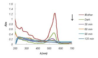
**Fig. 6.** Photodegradation of RB on bare ZnO/SiO<sub>2</sub> photocatalyst at pH=5.
