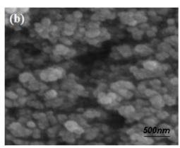
Fig. 3. SEM images of (a) bare ZnO, and (b) Pt- ZnO/SiO<sub>2</sub> nanoparticles.
