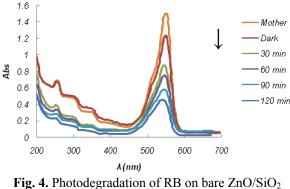
Fig. 4. Photodegradation of RB on bare ZnO/SiC photocatalyst at pH=3.
