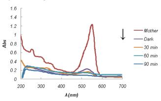
**Fig. 8.** Photodegradation of RB on Pt-ZnO/SiO<sub>2</sub> photocatalyst at pH=5.
