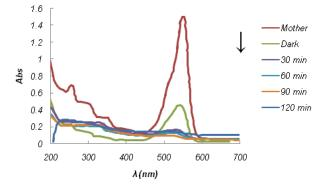
**Fig. 9.** Photodegradation of RB on Pt-ZnO/SiO<sub>2</sub> photocatalyst at pH=5 (under visible light).
