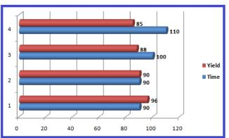
**Fig. 2.**The synthesis of triarylmethanes in the presence of reused [Msim]AlCl4 under solvent-free conditions at 70°C.
