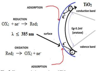
Fig. 5. Photo - catalytic procedure of TiO<sub>2</sub>
