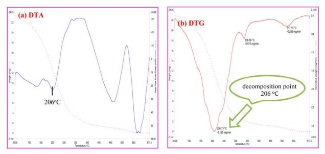
Fig. 3. (a) TG, DTA and (b) DTG of morpholinium glycolate.
